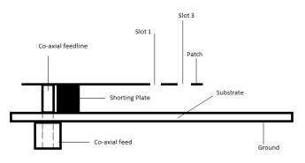
**Fig -3**: Side-view of PIFA with slots
