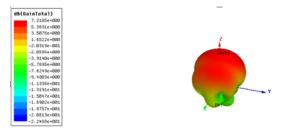
Fig -13. Radiation pattern for 2.2GHz for three slots PIFA
