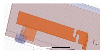
Fig -9: Top view of two slots PIFA
