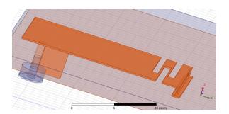
Fig.12 Top view of three slots PIFA
