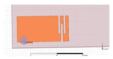
Fig -5: Top-view model of PIFA with slots
