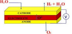
Fig.1. Scheme of a SOFC cell operating under electrolysis mode
