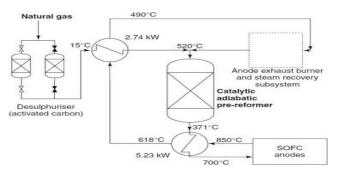
Fig. 2. Pre-reformer system devised for a Siemens 50-kW SOFC demonstration [6].
