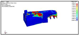
Fig -11: Strain plot of modified model.
