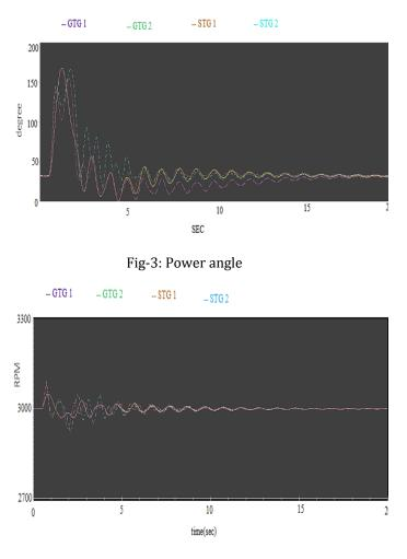
Fig-4: Generator speed
