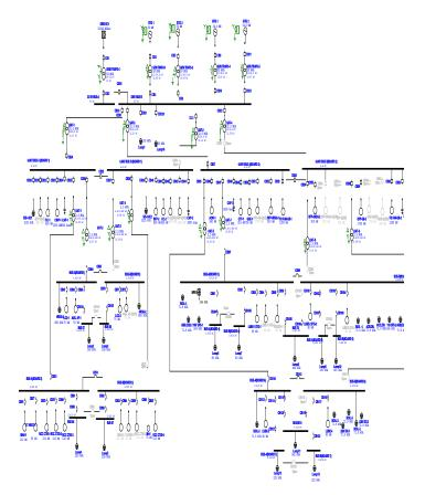
Fig-1: Single line diagram of combined cycle power plant
