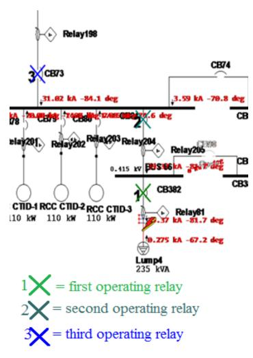
Fig-6: Relay co-ordination of the system
