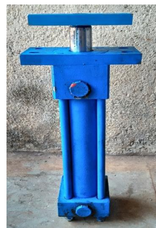
Fig -2: Double acting Hydraulic Cylinder
