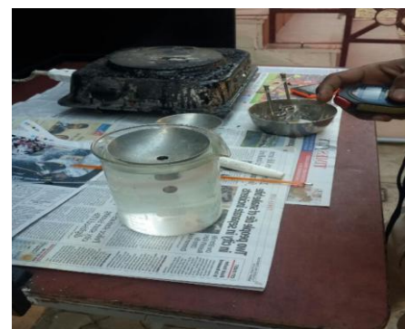
Fig- 3: Experimental setup for float test
