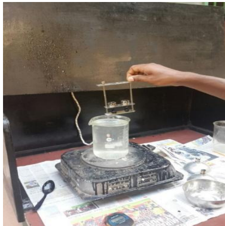
Fig-4: Experimental setup for softening point test
