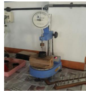
Fig -1: Experimental setup for penetration test
