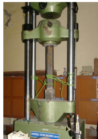
Figure-3 Testing of axial compression of I-section column
