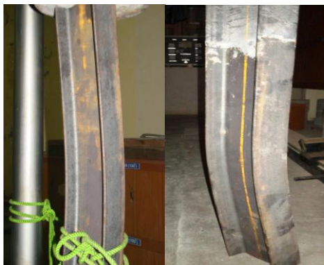
Figure-6 Deformed shape of I-Section
