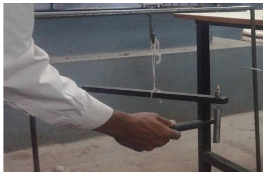
Fig.2.6 Accelerometer, impact hammer with carbon fiber sample rod while experimentation
