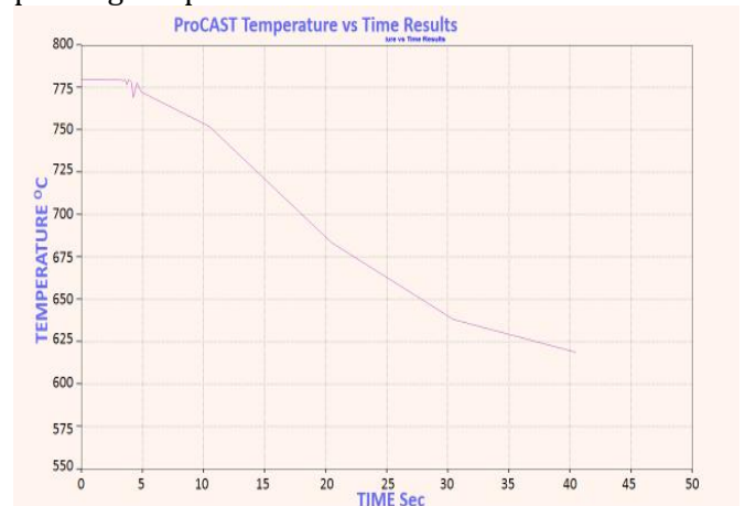
Figure. (2a): Temperature – time curve for 750 o C pouring temperature at location – 1.
