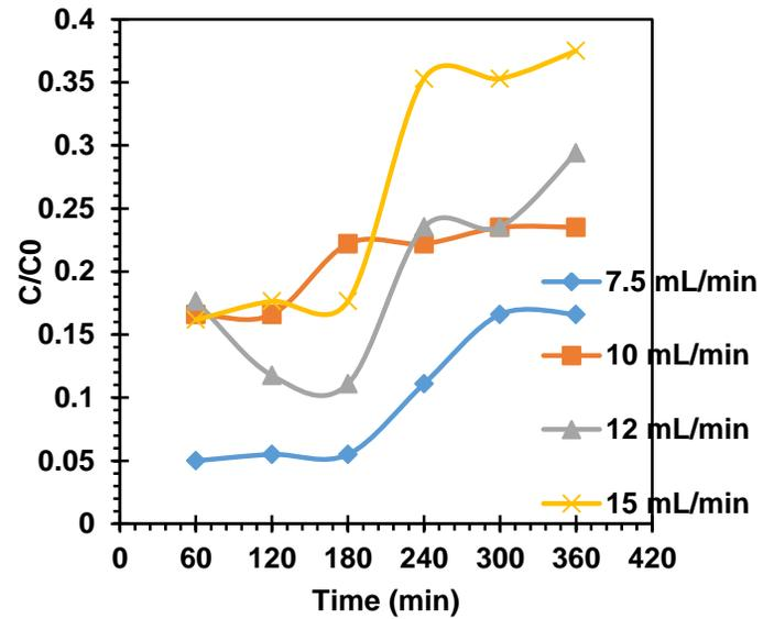
Chart 3 Breakthrough Curves for Effect of Flow Rate at Critical Depth for Synthesized Zeolite  $Z_1$ .
