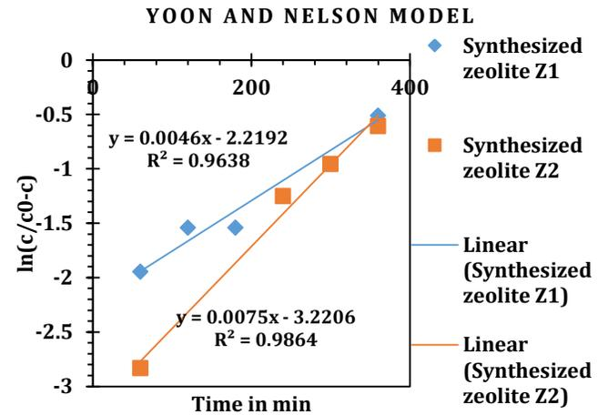
Chart 7 Yoon and Nelson model for synthesized zeolite Z<sub>1</sub> and Z<sub>2</sub>.
