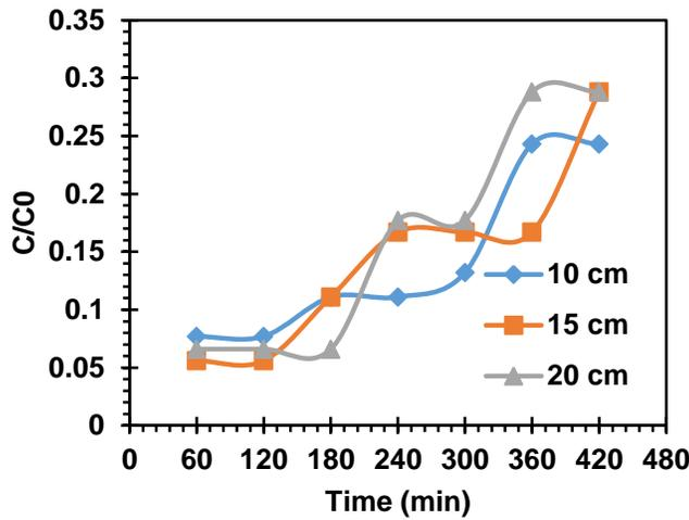
Chart 1 Breakthrough Curves at Different Bed Depths for Synthesized Zeolite  $Z_1$  at a Flow Rate of 15 mL/min.
