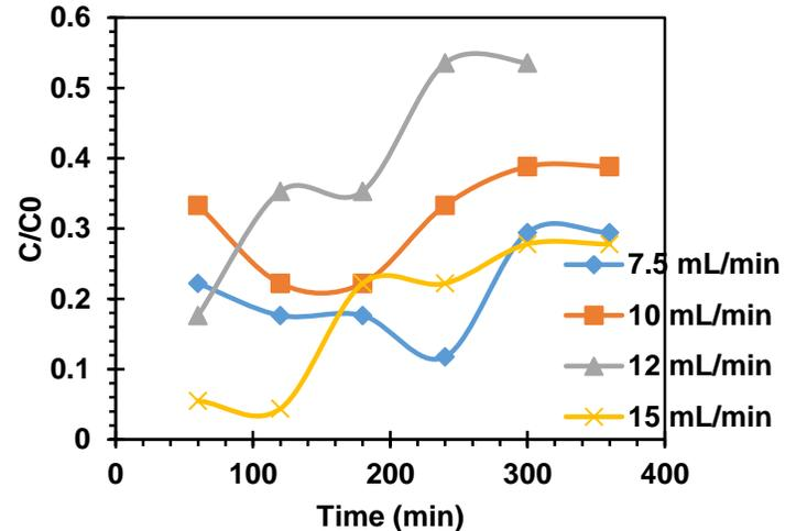
Chart 4 Breakthrough Curves for the Effect of Flow Rate at Critical Depth for Synthesized Zeolite  $Z_2$ .
