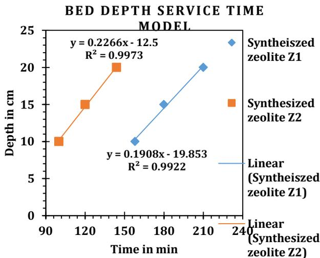
Chart 5 Bed depth service time model for synthesized zeolite  $Z_1$  and  $Z_2$ .
