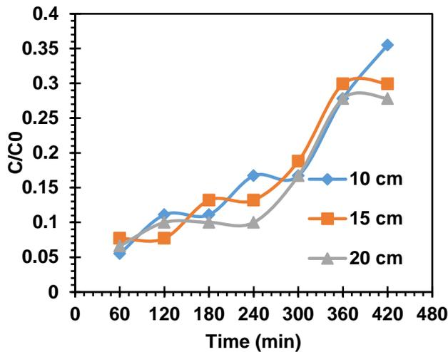
Chart 2 Breakthrough Curve at Different Bed Depths for Synthesized Zeolite  $Z_2$  at a Flow Rate of 15 mL/min.
