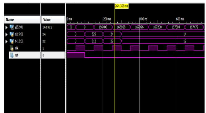
Fig. 11. Simulation of MAC unit hybrid CSKA
