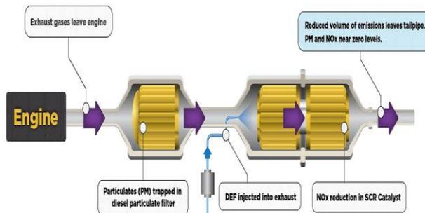
Fig1. Selective catalytic reduction process.
