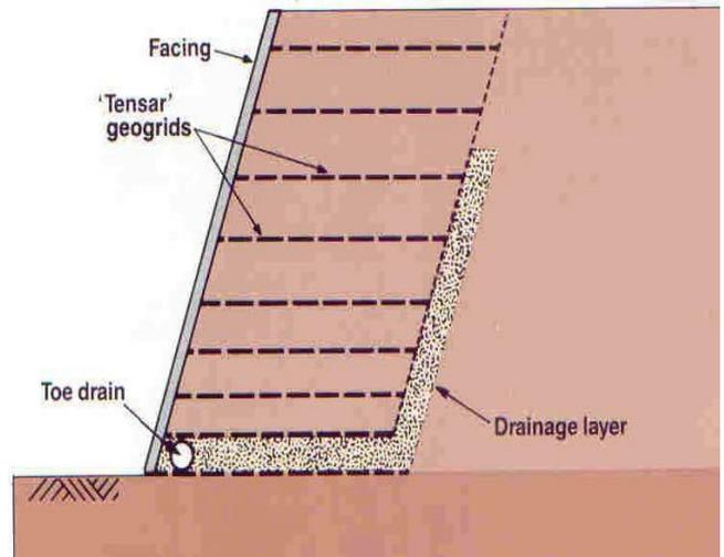
Fig -8: Facing with drainage
