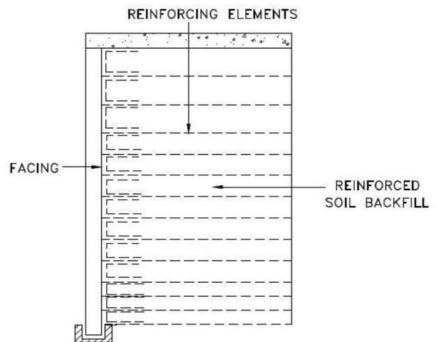
**Fig -1:** Components of reinforced earth structure
