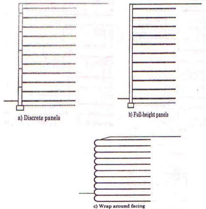
Fig -6: Common facing used with structure
