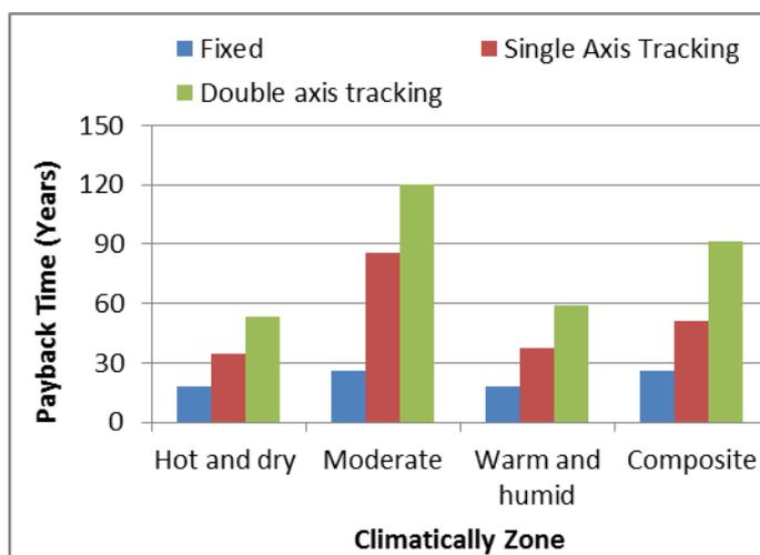
Fig .3 Comparison of Payback time (PV area 90 m<sup>2</sup>)
