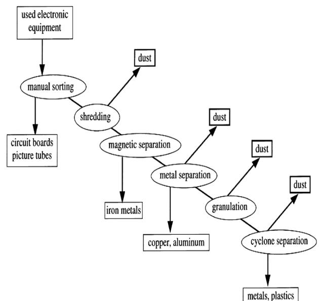
Fig 4 Generic e-waste treatment flow diagram
