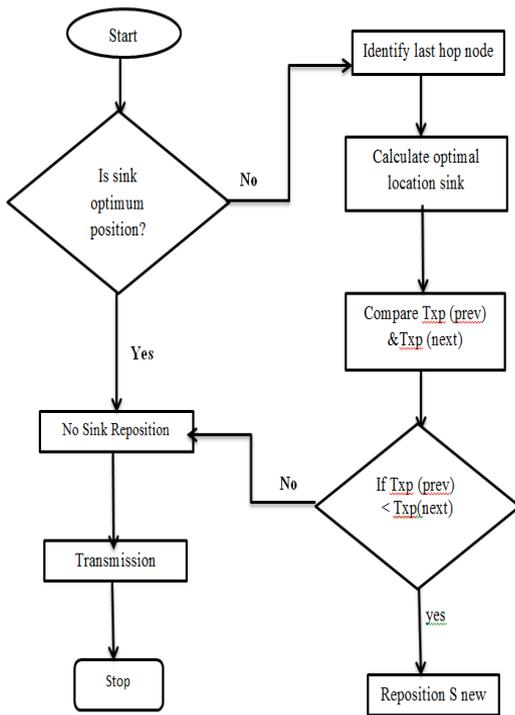
Figure 2 Flow chart of sink Reposition
