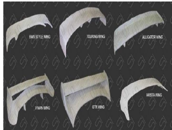
Figure 5 Different types of spoilers available in market.
