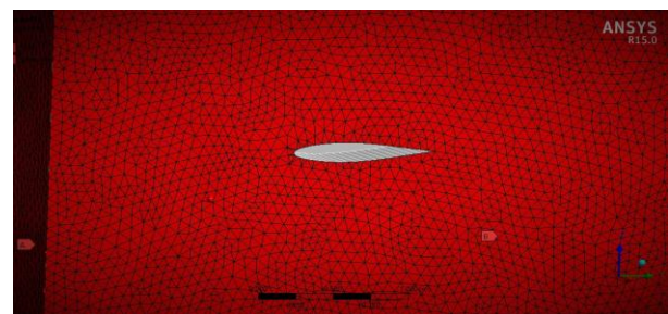
Fig-7: 3D Meshing of Baseline Aerofoil
