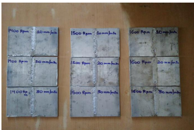
Photo-3: Aluminium Plates after FSW
