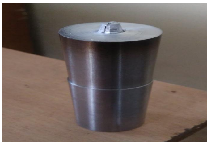
Photo-4: FSW Tool after welding
