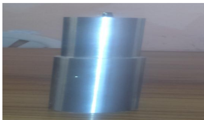
Photo-1: Actual FSW Tool before welding
