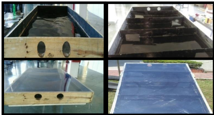
Fig-2: Construction of solar collector
