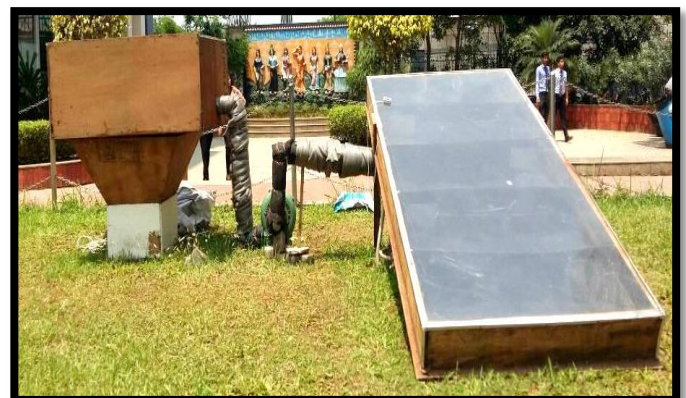
Fig-5: The experimental Setup of the Solar Dryer
