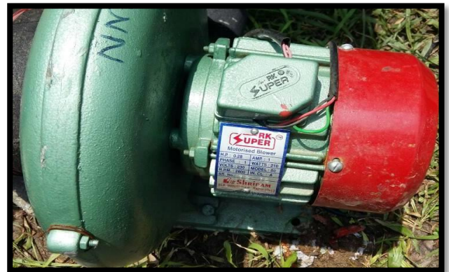
Fig-4: Air Blower
