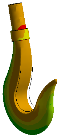
Figure 12: Maximum principal stress in crane hook is 297.95 mpa
