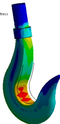
Figure 8: max equivalent stress in crane hook is 310.45 mpa
