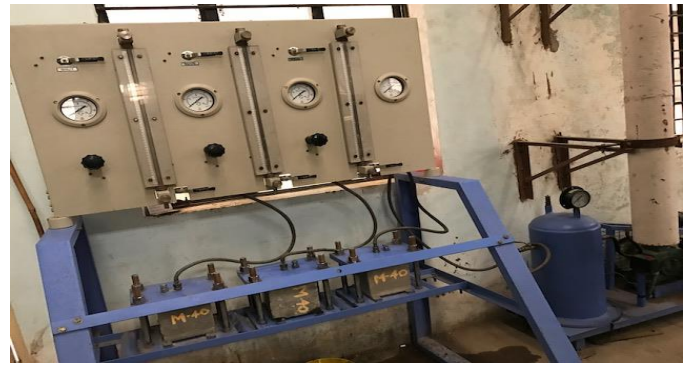
Fig- 8 Water Permeability apparatus setup
