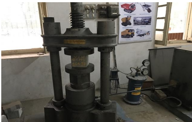
Fig- 3 test setup for cube under UTM
