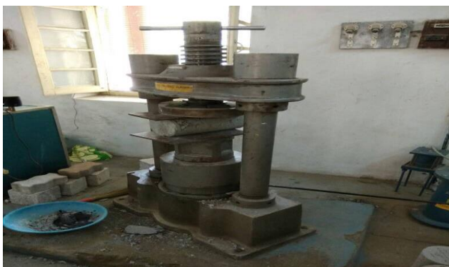
Fig-4 test setup of cylinder under UTM
