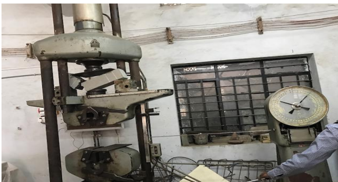
Fig- 7 Failure pattern of beam under UTM
