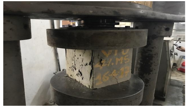
Fig- 4 failure pattern of cube under UTM
