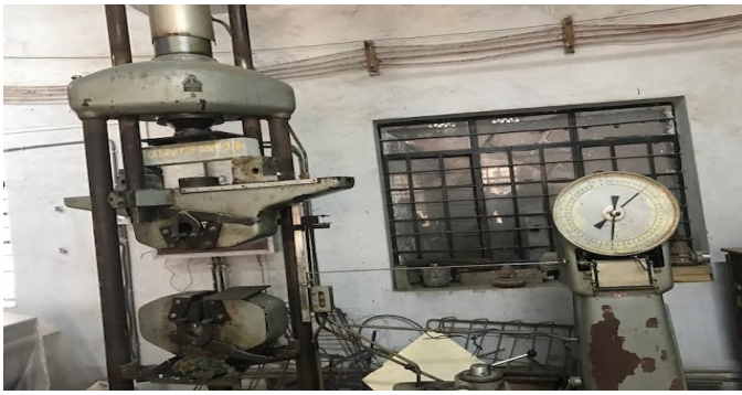
Fig- 6 Test setup of beam under UTM
