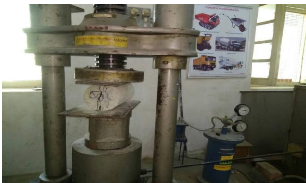
Fig- 5 failure pattern of cylinder under UTM
