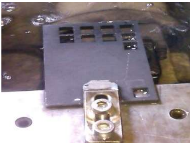
Fig -3: The cutting of graphite plate by WEDM
