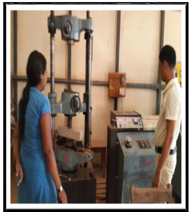
Fig -2: Flexural Testing
