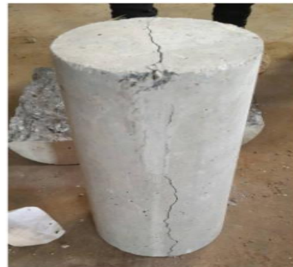
Fig -4: Failed Specimen
