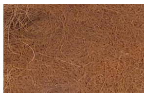
Fig 2 :-Rubberized coir sheet
