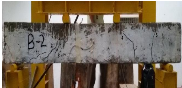
Fig 12:- cracked pattern of beam
