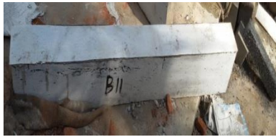
Fig 9:- Beams are wrapped with PP sheets
