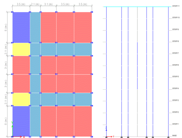
Fig-3 showing details of regular building with floating column (plan and elevation) of model-2
