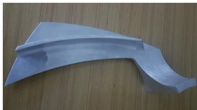
Fig.14: Impeller sector manufactured with Al25Zn material
