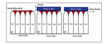
**Fig -8**: Schematic Representation of filling process of epoxy-based composites.[13]
