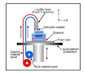
Fig -1: Schematic Representation of FDM Process
