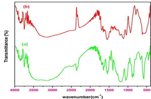
**Fig - 1:** FTIR spectra of (a) PPy and (b) PPy/Sn
