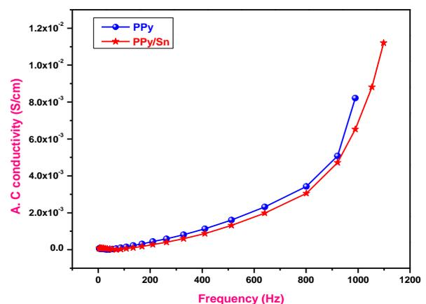
Fig - 4: A.C Conductivity of (a) PPy and (b) PPy/Sn
