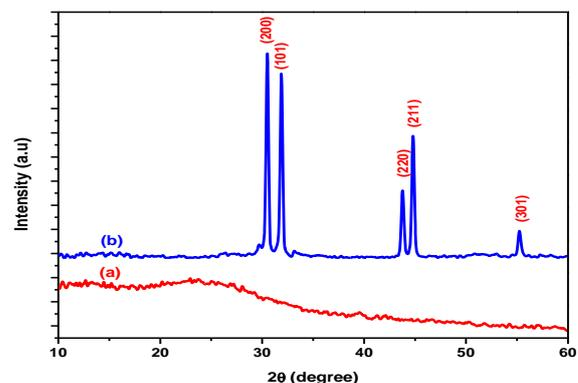
**Fig - 2:** XRD spectra of (a) PPy and (b) PPy/Sn
