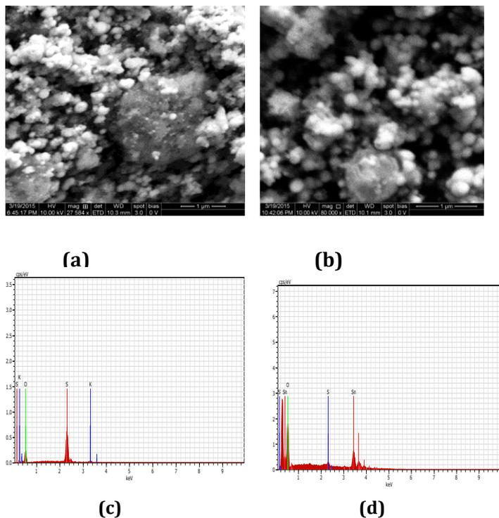
Fig - 3: FESEM with EDX image of (a & c) PPy and (b & d) PPy/Sn
