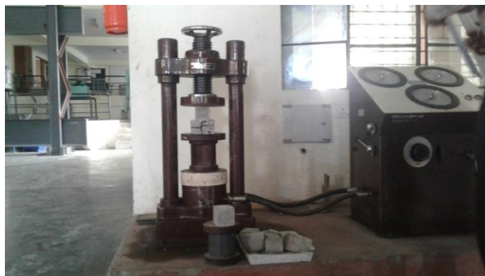
Figure – 5.1 Compressive tests on concrete cube.
