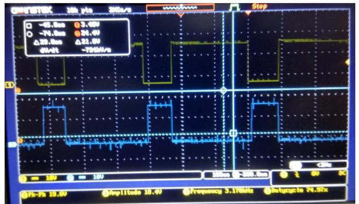
Figure 8 GATE SHOOT THROUGH WAVEFORM
