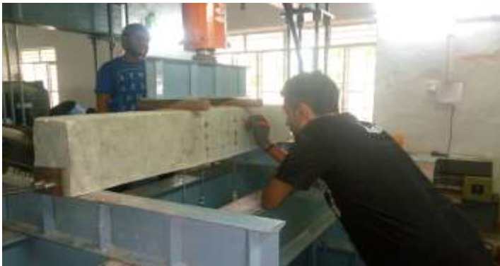
Fig 6:- Deflected shape of Post Tensioned Beam
