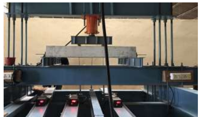
Fig 5:- Test setup for Post Tensioned Beam
