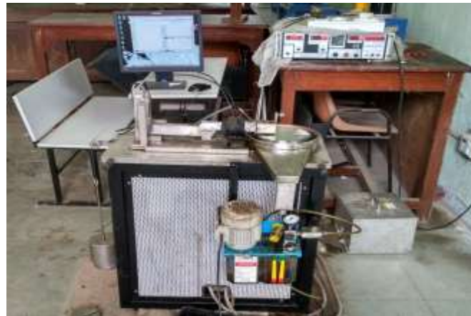
Figure 6: Schematic Setup of Pin ON Disc Machine
