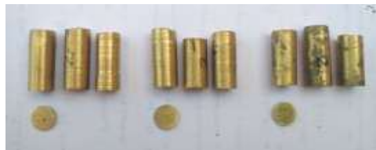
Figure 2: Pin produced after machining
