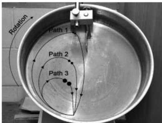
Fig-2: Growing path of pellets
