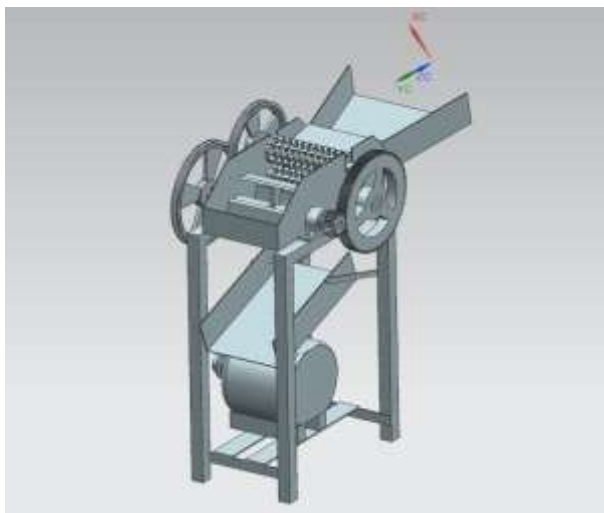
Fig.5 Assembly of Chaff Cutter Machine
