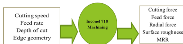
Fig 4. Interrelations between the processing conditions and the output variables
