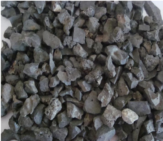
Fig - 2: Air cooled ferrochrome slag
