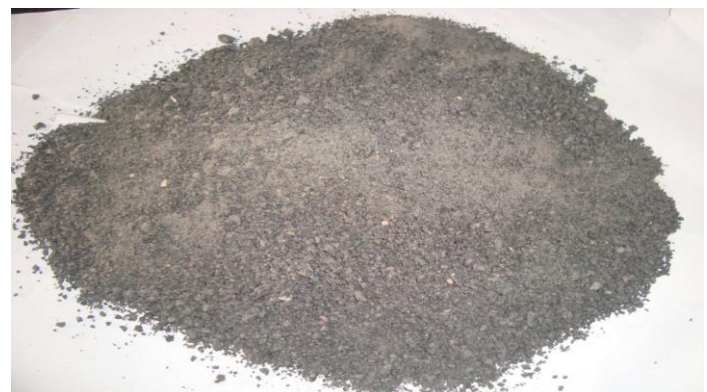
Fig - 1: Water cooled ferrochrome slag
