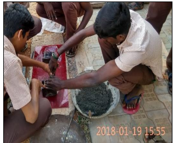
Fig -3: Casting of cubes
