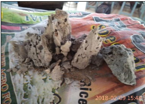
Fig -6: Broken cubes fragments showing inner pores
