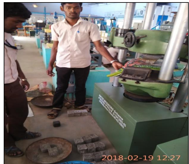
Fig -4: Compression test on cubes
