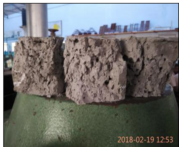
Fig -5: Broken cubes showing inner pores
