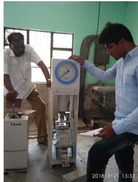
Fig-2: Flexural strength testing
