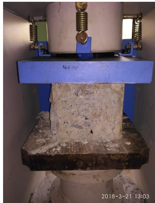
Fig-1: Compressive strength testing
