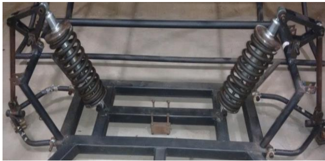
Fig -32: Rear suspension geometry actual assembly
