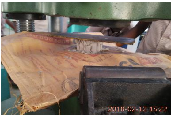
Fig -4: After compression strength test
