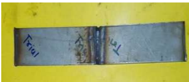
Fig -3: Welded Specimen
