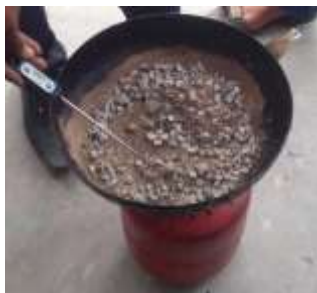
Fig -5: Heating of Aggregates Fig -6: Mixing of Bitumen
