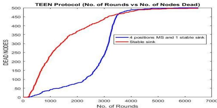
**Fig - 3:** Comparison of dead nodes with stable and mobile sink in TEEN protocol
