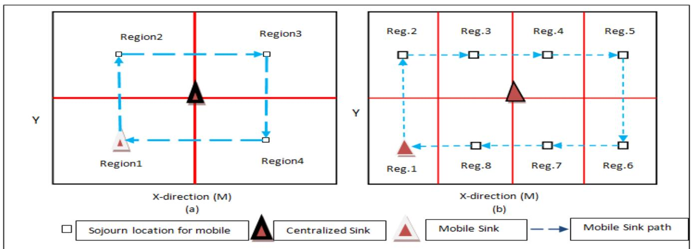
Fig - 2 (a) Sensor network with 4 sojourn locations Mobile Sink (b) Sensor network with 8 sojourn locations Mobile Sink
