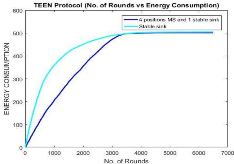
**Fig - 6:** Comparison of amount of energy consumed per round with stable and mobile sink in TEEN protocol
