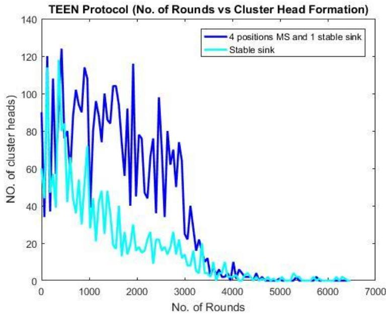
Fig - 4: Comparison of number of cluster head over number of rounds with stable and mobile sink in TEEN protocol
