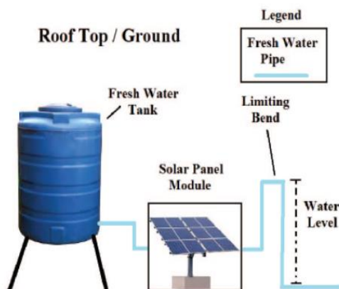
Fig -3: Solar Panel Cooling System
