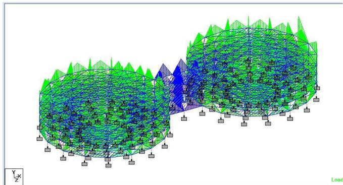
Fig -4: Live load diagram
