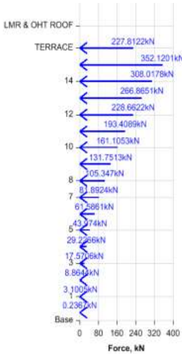
Fig 5.13.1 Shows weak storey in X-direction
