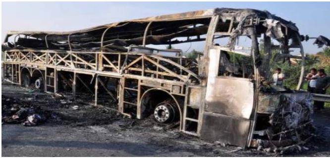
Fig 1.3: Rollover and fire failure of the bus structure
