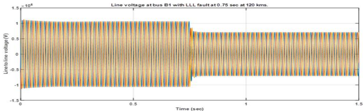
Figure 3.1: Three phase sending end line voltage in transmission circuit (V) at bus B1 with a LLL fault in transmission circuit at 0.75 sec at 120 kms.
