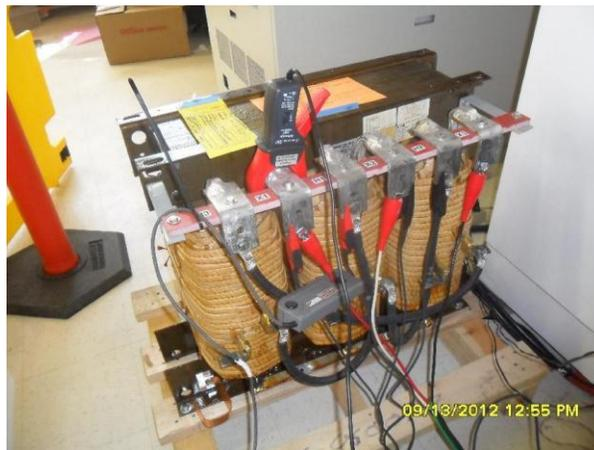
Figure 1.9: Snap picture of a 3-Phase 100KVA Transformer under test.
