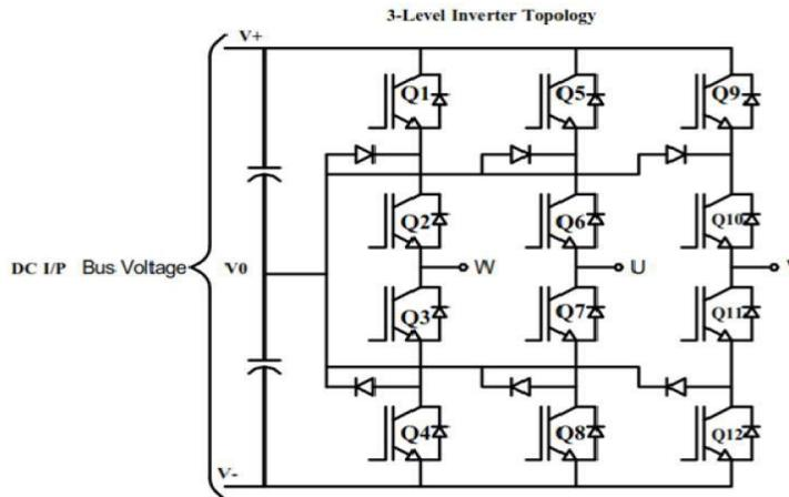
Figure 1.6 3-level 3-phases Inverter Topology [31]
