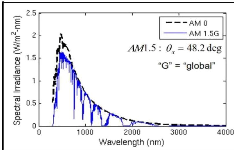
Figure 1.2 Solar Radiation Air Mass standards and corresponding Latitude [22]
