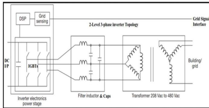
Figure 1.5 2-level 3-phase Inverter Topology [18]
