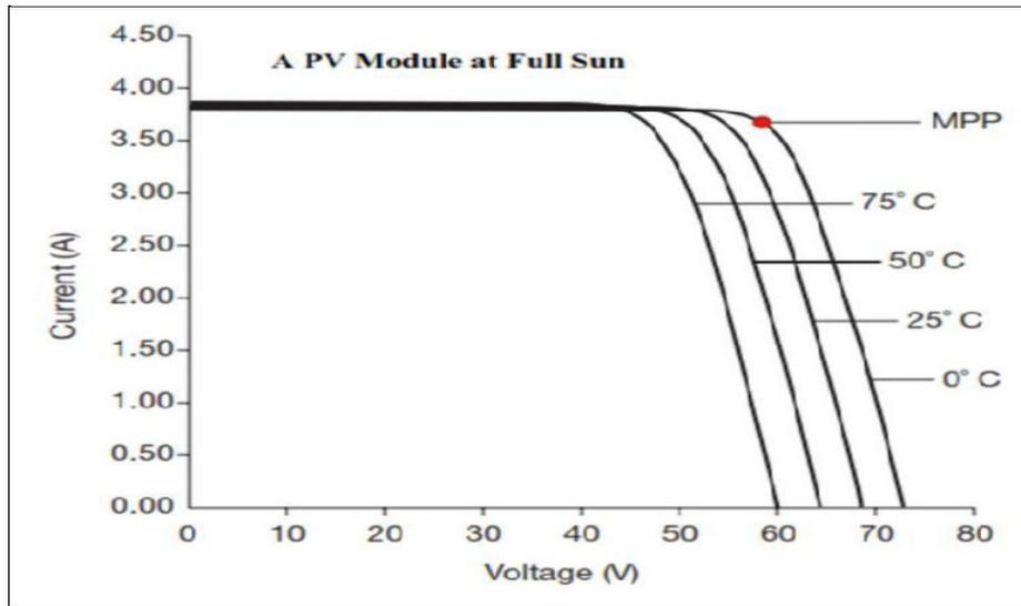
Figure 1.7 MPP on IV-Curve of a PV Module. [18]
