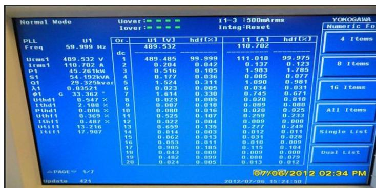
Figure 1.8 Harmonics of a 3-phase Grid-tied Inverter system.
