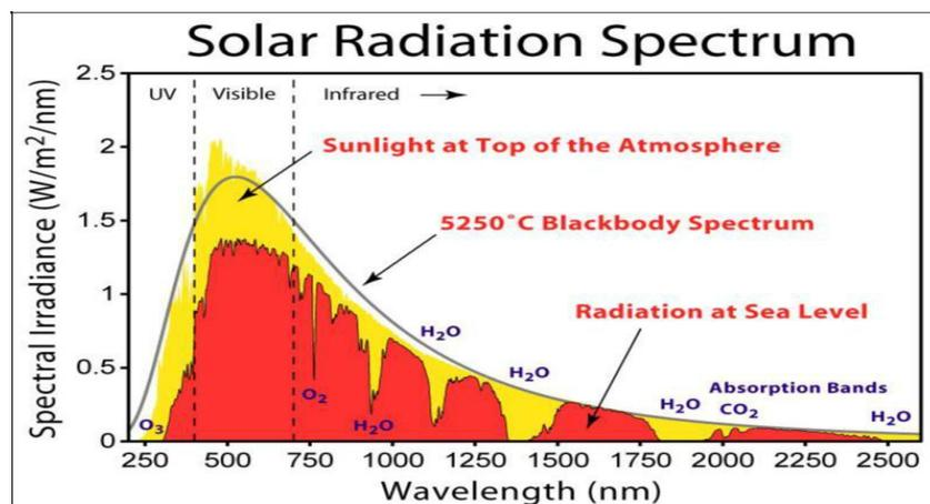
Figure 1.1 Solar Radiation Spectrums [2], [17]
