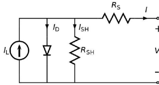
Figure 1.4 Practical Solar Cell Equivalent circuits. [17]
